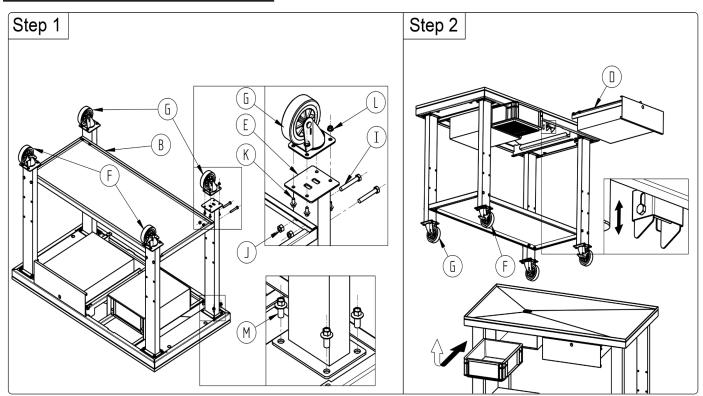
NOTE: The height of the shelf (item B), can be adjusted to any one of the three locations using the nuts and bolts (item I and item J).
