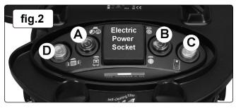
6.1.4. If the exhaust air speed drops below 20m/sec warning light "C" 📓 illuminates in accordance with IEC/EN60335-2-69.
