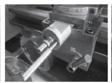
2. Remove the dial bracket and take out the cross slide feed screw.
