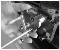
5. Assemble the digital readout box (part no.1) onto the bracket, then fit the assembled transition shaft and ball handle into the leadscrew. Slightly adjust the transition shaft to make it work properly with the leadscrew. Finally, tighten with two M3 x 25mm screws (part no.8).
