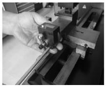
7. Assemble the digital readout box (part no.1) onto the bracket, then fit the assembled transition shaft and ball handle into the lead screw. Slightly adjust the transition shaft to make it work well with the leadscrew. Finally tighten with two M3 x 25 screws (part no.8).
