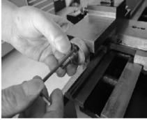
2. Loosen the screws. Remove the dial bracket and take out the compound feed screw.
