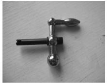
4. Assemble the transmission shaft (part no.4) onto the dismantled ball handle.
