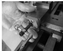
6. Refit the dismantled, original M4 x 12 screws. Take out the transition shaft again.
