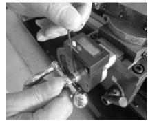
6. Make the final adjustment for free movement of the handle with little drag. Lock the small screws.
