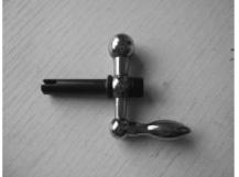
5. Assemble the transition shaft (part no.5) onto the dismantled ball handle.
