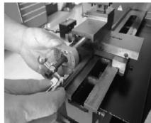
4. Use the transition shaft to push the assembled compound feedscrew and bracket into the compound slide.
