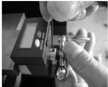
8. Make the final adjustment for free movement of the handle with little drag. Lock the small screws.
