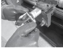
1. Remove the screw securing the cross slide handle. Remove the ball handle, spacer and dial.
